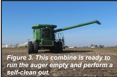
**Figure 3.** This combine is ready to run the auger empty and perform a self-clean out.
